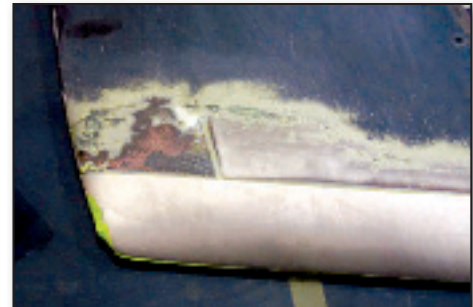
Rotorblade Damage by Erosion
