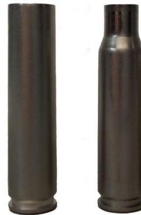
Lighter-weight stainless steel metal injection molded small caliber ammunition cases. (Photo credit: U.S. Army)
