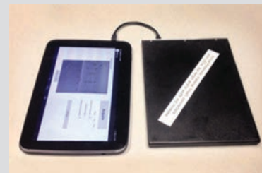
6"x6" flexible digital X-ray Panel — Android OS
