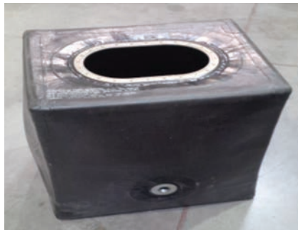
Notional improved aviation fuel bladder
