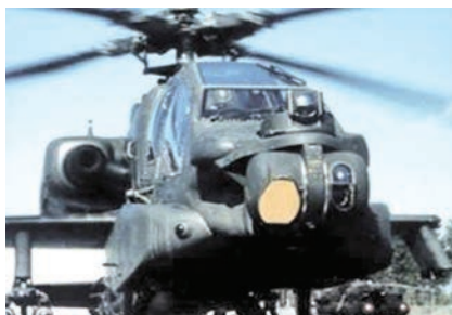
PNVS Turret Drive System AH-64 Apache
