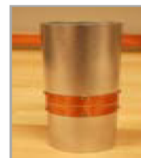
Two Piece Molded Conformal Antenna
