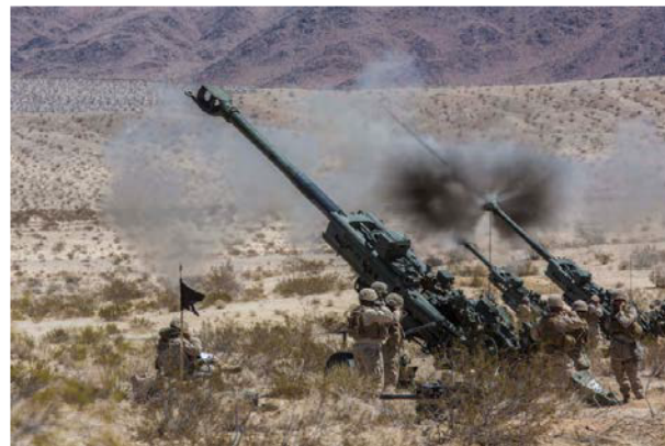
M795 projectile fired from a M777A2 Howitzer
