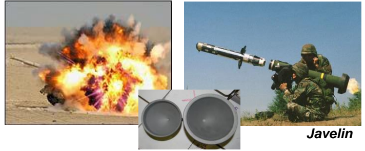
Near Net Shape Warhead Preform vs. Normal Preform
