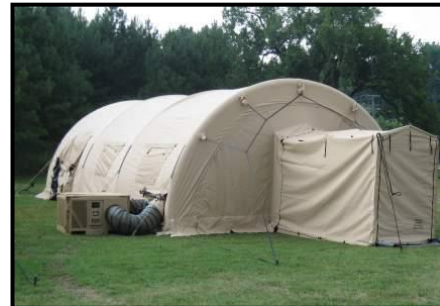
Tent, Extendable, Modular, Personnel – Air Supported (TEMPER - AS)
