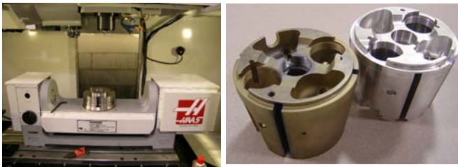
Haas VF-3 machine tool with rotary tilt table (left). Processed bottom plate (right).
